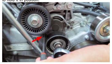
90. Using a 12mm and 14mm socket, remove the bolt securing the alternator to the alternator bracket and the bolt securing the alternator bracket to the engine.
