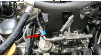
123. Connect the low pressure fuel feed line to the driver side fuel rail. Verify the lock is engaged by gently tugging on the fuel line.
