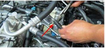
48. Using a 10mm socket, unbolt the throttle body from the intake manifold. Position the throttle body towards the front of the vehicle but do not disconnect the coolant lines at this time.
