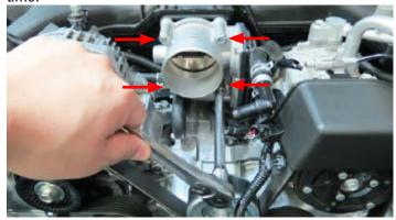
49. Using needle nose pliers, remove the engine harness from the rear passenger side manifold runner. Using a 12mm socket, remove three (3) bolts securing the passenger side of the manifold to the cylinder heads.
