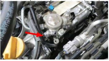
62. Install the low pressure fuel feed line onto the banjo fuel fitting. *TIP: Fuel line will be the one closest to the mechanical fuel pump.*
