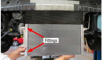
97. Align the A/C condenser and the LTR. Using a 10mm socket, secure the LTR to the A/C condenser using the factory hardware.
