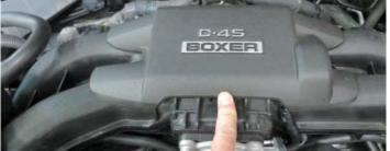
26. Unplug the MAP sensor connector located on top of the driver side intake manifold runner.
