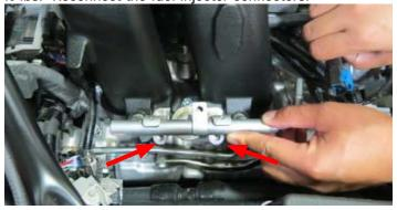
120. Connect the passenger side fuel crossover line to the fuel rail and engage the blue locking clip.
