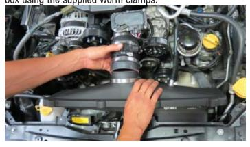
160. Clock the worm clamps to position the screws away from the A/C compressor belt/pulley. Double check that there is at least 6mm clearance between the coolant line on the throttle body and the belt on the AC compressor pulley.
