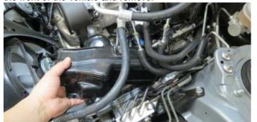
41. Release the blue locking clip from the fuel crossover and disconnect the crossover line from the driver side fuel rail.
