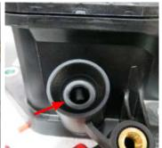
36. Using a 10mm socket, remove the EVAP line support bracket from the driver side manifold.
