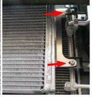
98. Using a 14mm socket, remove the two front lower bolts securing the A/C compressor to the engine.
