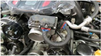
132. Using a factory hose clamp, secure the throttle body coolant outlet hose to the throttle body outlet fitting.
