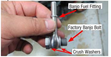
61. Carefully install the banjo fuel fitting assembly onto the mechanical fuel pump. Clock the fitting to the 1 o'clock position and torque the banjo bolt to 23 ft.lbs (31 N.m).
