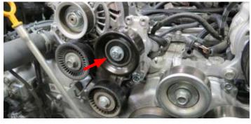
93. Rotate the tensioner clockwise using a 14mm socket and remove the small screw driver holding the tensioner open.
