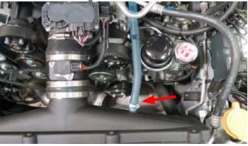
163. Using the 3/4" Hose Clamp and M5 x 8mm Button Head Flange bolt from Bag #4, secure the driver side PCV hose to the PCV support bracket.
