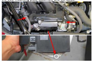
33. Place a rag under the fuel crossover line to absorb any fuel that make leak. Release the blue locking clip located on the fuel crossover line and carefully remove the fuel crossover line from the passenger side fuel rail.
