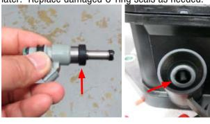
45. Using a Subaru fuel line removal tool #42099AE000, or equivalent, remove the low pressure fuel feed line from the driver side fuel rail assembly. Remove fuel rail assembly and set aside as it will be reused later.
