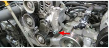
92. Using the M8 x 170mm bolt and M8 washer from Bag #1, secure the supplied pulley and the FEAD bracket to the top alternator bracket bolt provision. Torque the M8 bolt to 18 ft-lbs and the M10 bolt to 22 ft-lbs.
