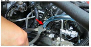
87. Connect the supplied 29" EVAP hose to the factory EVAP hard line. Route the hose towards the A/C compressor and under the driver side PCV hose. Connect the other end of the EVAP hose to the EVAP solenoid fitting farthest from the connector. Secure the EVAP hose to the solenoid using a 5/8" hose clamp from Bag #4.
