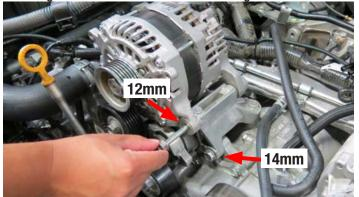
91. Position the supplied FEAD bracket onto the alternator mounting bracket. Using the M10 x 70mm bolt from Bag #1, loosely secure the FEAD bracket to the lower alternator bracket bolt provision.
