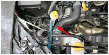
114. With the intercooler hoses properly secured, reposition the supercharger rearwards. Noting the orientation of the factory fuel crossover line, carefully snake the line under the supercharger nose, behind the alternator and out in front of the passenger side runner.
