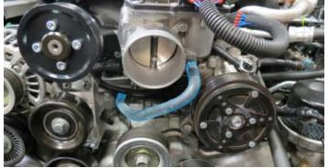
133. Using a 14mm socket, rotate the belt tensioner clockwise and install the supplied drive belt using the routing diagram below.
