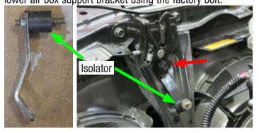
146. Install the 5/16" grommet and grommet sleeve from Bag #3 onto the left air box bracket.
