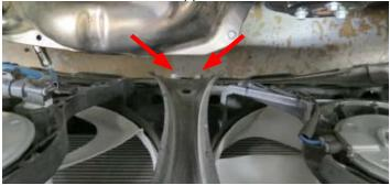
145. Install the isolator onto the lower air box support bracket. Using a 10mm socket, remove the bottom bolt securing the hood latch assembly and install the supplied lower air box support bracket using the factory bolt.
