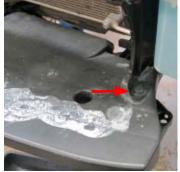
15. Connect a rubber hose to the drain barb located on the petcock. Place the other end of the hose into a drain bucket and loosen the petcock to drain the radiator fluid. *TIP:* Rubber hose is not require but will limit spillage and cleanup.
