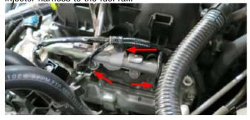
43. Using a 12mm socket, remove two (2) bolts securing the driver side fuel rail to the manifold. Remove fuel rail assembly and move aside.
