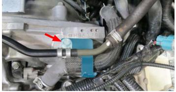
84. Remove the EVAP solenoid from the bottom of the factory intake manifold.
