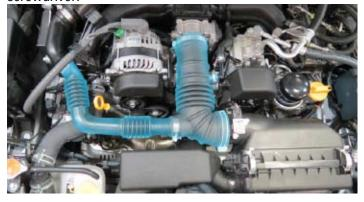
18. Using a 10mm socket, remove two (2) bolts securing the noise generator assembly to the ECU mounting plate. Disconnect the noise generator hose from the firewall and plug the hole with the 1" sheet metal plug from Bag #4.
