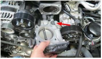
130. Using the factory throttle body bolts, secure the throttle body to the supercharger with the connector oriented upwards.
