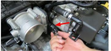
28. Remove the PCV and brake booster hoses attached to the top of the intake manifold. *NOTE: Automatic applications will have a PCV hose and a rubber cap.*
