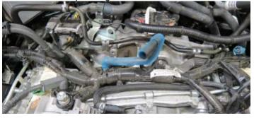
68. Install the  $90^{\circ}$  end of the supplied passenger side PCV hose onto the passenger side PCV fitting. Secure hose with a 5/8" hose clamp from Bag #4.
