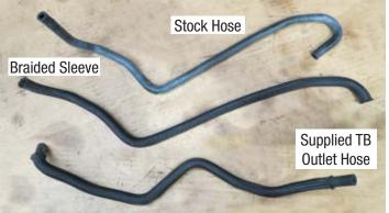
71. Install the straight end of the supplied throttle body outlet hose onto the driver side cylinder head coolant fitting and secure with a factory hose clamp. Route the hose under the engine harnesses and towards the front of the vehicle.
