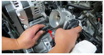
65. Remove the throttle body coolant hose from the coolant crossover using a hose clamp tool, or equivalent,.
