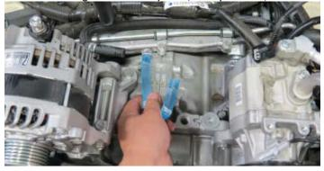
66. Install the straight end of the supplied throttle body inlet hose to the coolant crossover and secure with the factory hose clamp.
