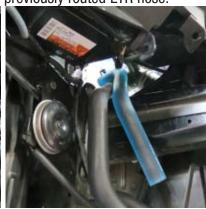
111. Using a 10mm socket, remove the bolt securing the front of the fuse box. Insert the surge tank bracket under the fuse box and secure the bracket along with the fuse box with the factory bolt.
