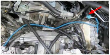
83. Using a 12mm socket, remove the bolt securing the brake booster hard line to the engine. Position the supplied EVAP bracket under the brake booster line and secure the EVAP bracket and brake booster line using the factory bolt.
