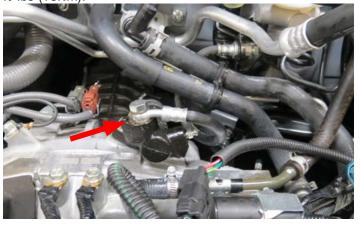
57. Fill the clutch reservoir to the MAX line with FMVSS No. 116 DOT3 brake fluid, or equivalent. *NOTE: During the clutch bleeding procedure, DO NOT let the clutch fluid in the reservoir go below the MIN line.*
