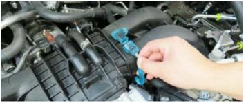
27. Disconnect the throttle body connector from the throttle body.
