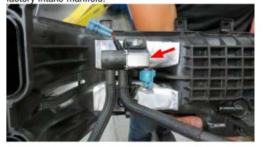
85. Secure the EVAP solenoid to the EVAP bracket using the factory nut. Connect the EVAP extension to the EVAP connector located on the water pump harness.
