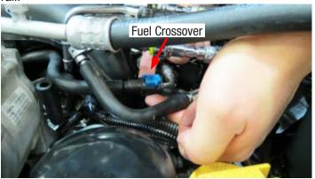
42. Unplug the driver side fuel injector connectors. Using needle nose pliers, remove the plastic rivet securing the injector harness to the fuel rail.
