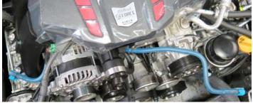
115. Snake the other end of the fuel crossover behind the A/C compressor and out in front of the driver side runner.
