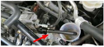
59. Using a 17mm wrench, remove the banjo bolt securing the low pressure fuel feed line to the mechanical fuel pump. Remove the fuel feed line as it will not be reused.
