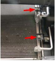
96. Remove the protective covers on the Low Temp Radiator (LTR) fittings. Carefully position the LTR, with the fittings pointing towards the passenger side of the vehicle, onto the A/C condenser mounting brackets.
