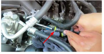
47. Using pliers, remove the rubber EVAP line from the hard line assembly.
