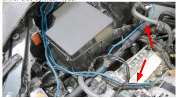
81. Connect the +12V Constant Power terminal to the positive stud on the battery terminal. Secure the Fuse to existing wire looms with wire ties.
