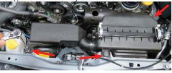
21. Using a 10mm socket, remove two (2) bolts securing the lower air box assembly and remove.
