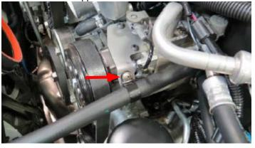
164. Connect the male MAF sensor connector, on the supplied TMAP harness, to the factory MAF sensor connector. Connect the female MAF sensor connector to the factory MAF sensor.
