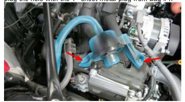
19. Remove the MAF harness from the A/C compressor pulley cover. Unplug the MAF sensor and remove it from the air box assembly using a small Phillips screwdriver. Place the MAF sensor in a clean area as it will be reused later.
