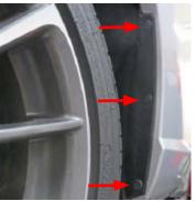
11. Carefully remove both side marker lenses by gently pulling out the upper corner of the lenses. Unplug the bulb assemblies and remove. *Tip: Lenses are secured with three* (3) metal clips pointed out by the red arrows.
