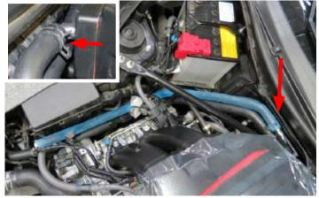
109. Attach the supplied surge tank to the other end of the Intercooler-to-Surge Tank hose and secure it with a 3/4" hose clamp from Bag #2.
