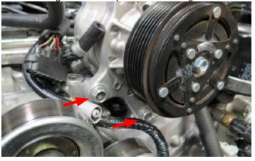
99. Using a 14mm socket, remove the rear A/C compressor bolt and carefully position the compressor forward. *NOTE: DO NOT remove the A/C lines as you will purge all of the pressurized freon.*
