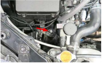
112. Using two (2) M6 x 10mm bolts from Bag #2, secure the surge tank to the surge tank bracket.
