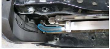
139. Route the W/P end of the hose down and over towards the water pump bracket.
