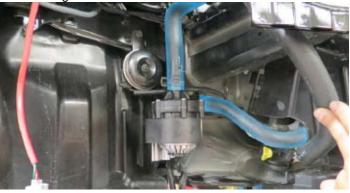
142. Route the water pump connector, from the previously installed water pump harness, down towards the water pump and connect it to the water pump. Secure the harness to existing wire looms and/or hoses.
