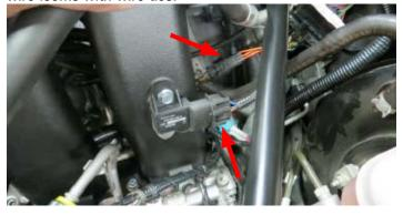
166. Using the push mount zip tie from Bag #2, secure the TMAP harness and the throttle body extension harness to the PCV support bracket.
