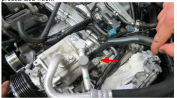
100. Using pliers, remove the driver side PCV hose located under the A/C compressor
