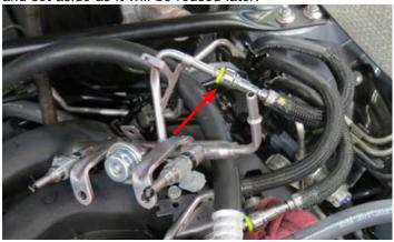
46. Using the fuel line removal tool, remove the other low pressure fuel feed line from the hard line leading to the mechanical fuel pump.
