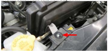
152. Use a M6 locknut and a M6 washer from Bag #4 to secure the front air box shroud to the isolator.
