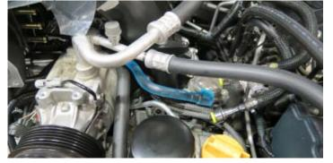
116. Realign the supercharger to the cylinder heads. Using two (2) M8 x 30mm bolts and one (1) M8 x 50 bolt, loosely secure the driver side runner to the cylinder head.
