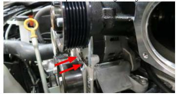
126. Connect the 45° end of the previously installed EVAP hose to the top nose fitting. Connect the RH/Passenger PCV to the bottom nose fitting. Manual applications will connect the Brake Booster hose to the center nose fitting. Automatic applications will remove the fitting plug from the stock intake manifold and install it to the center nose fitting.
