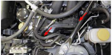
40. Carefully work the manifold support bracket towards the front of the vehicle and remove.
