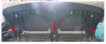
9. Use a panel puller to remove two (2) push fit rivets (red arrow) and a 10mm socket to remove two (2) bolts (green arrow) securing the fascia to the outer splash guards.
