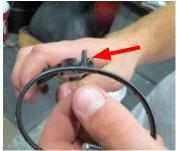
129. Install the O-ring seal onto the supercharger throttle body flange. Connect the throttle body coolant inlet hose to the inlet fitting and secure with the factory hose clamp.
