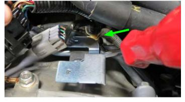
78. Relocate the transmission plugs and harness behind the heater hoses. Secure the harness and plugs to existing engine harnesses and A/C lines with wire ties as designated by the green arrows.
