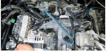
69. Using long needle nose pliers, remove the throttle body outlet coolant line from the driver side cylinder head fitting.
