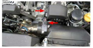
20. Using a 10mm socket, remove three (3) bolts securing the upper air box assembly and remove.
