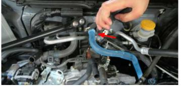
73. Using a hose cutter, or equivalent, cut approximately 1.75" from the passenger side heater hose.
