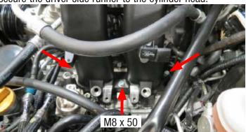
117. Using two (2) M8 x 30mm bolts and one (1) M8 x 50 bolt, loosely secure the passenger side runner to the cylinder head. Torque all six (6) bolts to 10 ft-lbs, starting with the center bolts and working outwards,
