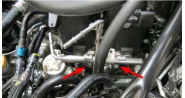
122. Connect the fuel crossover line to the driver side fuel rail and engage the blue locking clip.
