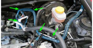
79. Mount the relay and ground strap on the water pump harness to the chassis bolt adjacent to the fuse box.
