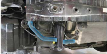
108. Install the Intercooler to Surge Tank hose onto the passenger side intercooler fitting and secure it with a 3/4" hose clamp from Bag #2. Position the ¾" hose clamp ears away from the brake lines. Route the hose along side the previously installed intercooler hose.
