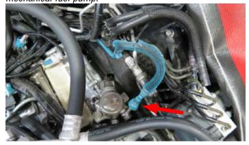
63. Using a hose clamp tool, or equivalent, remove the throttle body outlet hose from the throttle body outlet fitting.
