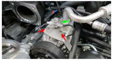
128. Remove the throttle body 0-ring seal from the factory manifold. Using side cutters, or equivalent, remove the tip from the 0-ring seal.
