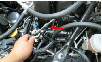
124. Reinstall the ECU mounting plate assembly using the factory hardware. Reconnect all ECU connections and reattach the engine harness and alternator harnesses to ECU plate.
