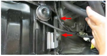
138. Using a 3/4" hose clamp from Bag #2, secure the LTR to W/P Hose to the top LTR fitting.
