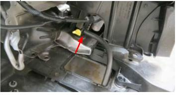
16. Using a hose clamp tool, or equivalent, remove the driver side PCV hose from the air inlet tube.
