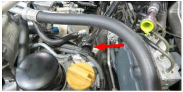
60. Assemble the supplied banjo fuel fitting from Bag #3 using the supplied 12mm crush washers and the factory banjo bolt.
