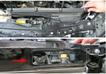
150. Use the M6 x 16mm Hex Flange bolt from Bag #4 to secure the front air box shroud to the upper radiator support. This is done from the inside of the air box by threading the bolt through the welded nut on the radiator support.
