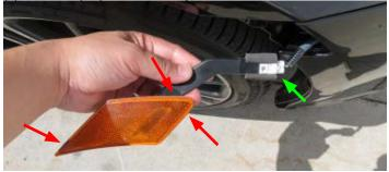
12. Using a panel puller, remove two (2) push pin rivets securing the front fascia to the fender.
