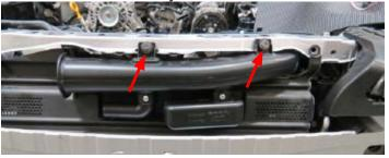
22. Using a panel puller, remove six (6) push pin rivets securing the radiator shroud and remove.
