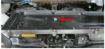
153. Re-secure the top radiator support using the factory hardware.
