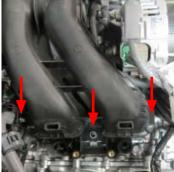
50. Using a 12mm socket, remove three (3) bolts securing the driver side manifold to the cylinder heads.
