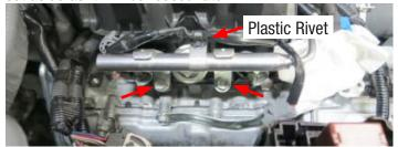
35. Inspect the fuel injectors to verify the O-ring seals are present. If not, the seals may be lodged inside the manifold injector provisions. Carefully use a small flat head screw driver to remove the seals and set them aside as they will be reused later. Replace damaged O-ring seals as needed.
