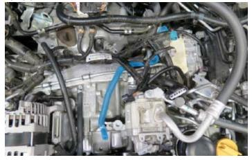
72. Using a hose clamp tool, or equivalent, remove the passenger side heater hose from the heater core fitting located on the firewall.
