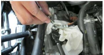
55. Remove the crush washer from the banjo bolt and from the bottom of the banjo end and discard.
