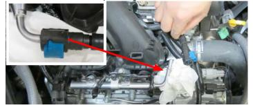
34. Remove the plastic rivet securing the fuel injector harness to the fuel rail using needle nose pliers, then unplug the passenger side fuel injector connectors. Using a 12mm socket, remove two (2) bolts securing the fuel rail to the manifold. Carefully remove the fuel rail assembly and set aside as it will be reused later.
