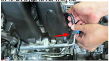
121. With the fuel injectors securely positioned on the driver side fuel rail, carefully install the fuel rail assembly with the injector connectors oriented outwards. Secure the fuel rails with the factory bolts and torque to 10 ft-lbs. Reconnect the fuel injector connectors.
