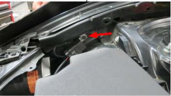
80. Route the Fuse Holder and Power +12V terminal, on the water pump harness, around the fuse box and towards the battery. Route the EVAP connector over towards the driver side cylinder head.
