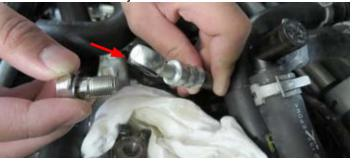
56. Route the clutch line underneath the heater hoses and orientate the clutch line so that it's pointing downwards and clocked towards the driver side of the vehicle. Secure the clutch line using the factory banjo bolt and the supplied 10mm crush washers from Bag #3. Torque banjo bolt to 13 ft-lbs (18Nm).
