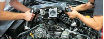
105. With the supercharger manifold properly positioned onto the cylinder heads, reinstall the A/C compressor and torque bolts to 22 ft lbs. TIP: The rear compressor bolt can be accessed through the opening of the driver side runner using a long extension and a universal socket.
