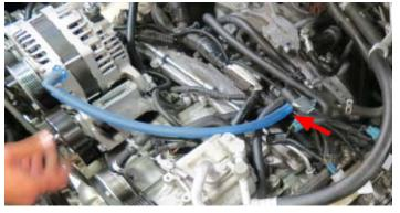
89. Rotate the tensioner clockwise using a 14mm socket. Insert a small screw driver into the grooves of the tensioner to hold it in position.
