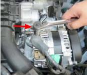
30. Remove the engine and alternator harness supports from the ECU mounting plate by pushing the locking tab in and pulling up.
