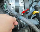
31. Remove all harness connectors from the ECU by depressing the locking tabs on the connectors and then rotating the connector levers outward until they release from the ECU.
