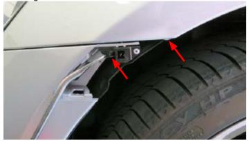
13. Unplug any front fog lights, if applicable, and carefully remove the front fascia.
