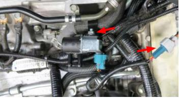
86. Using pliers, remove the factory EVAP hose from the hard line located in between the low pressure fuel feed lines.
