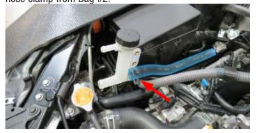
110. Using a 3/4" hose clamp from Bag #2, secure the 90° end of the Surge Tank to W/P hose onto the surge tank. Route the other end of the hose down towards the horn assembly along side the previously routed LTR hose.
