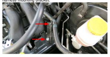
39. Using a 12mm socket, remove two (2) bolts securing the driver side manifold support bracket to the engine. NOTE: Removal of the driver side strut brace will simplify this procedure but is not required. Reinstall the strut brace once the driver side support bracket is removed.
