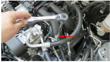
37. Disconnect the rubber EVAP hose from the EVAP hard line.
