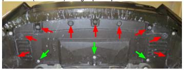
8. Using a 10mm socket, remove three (3) bolts securing the splash guard/fascia support.
