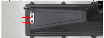
148. Install the supplied 5/16" grommet and grommet spacer onto the air duct of the front air box shroud.
