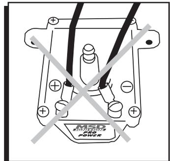
Figure 2 Incorrect Routing.
