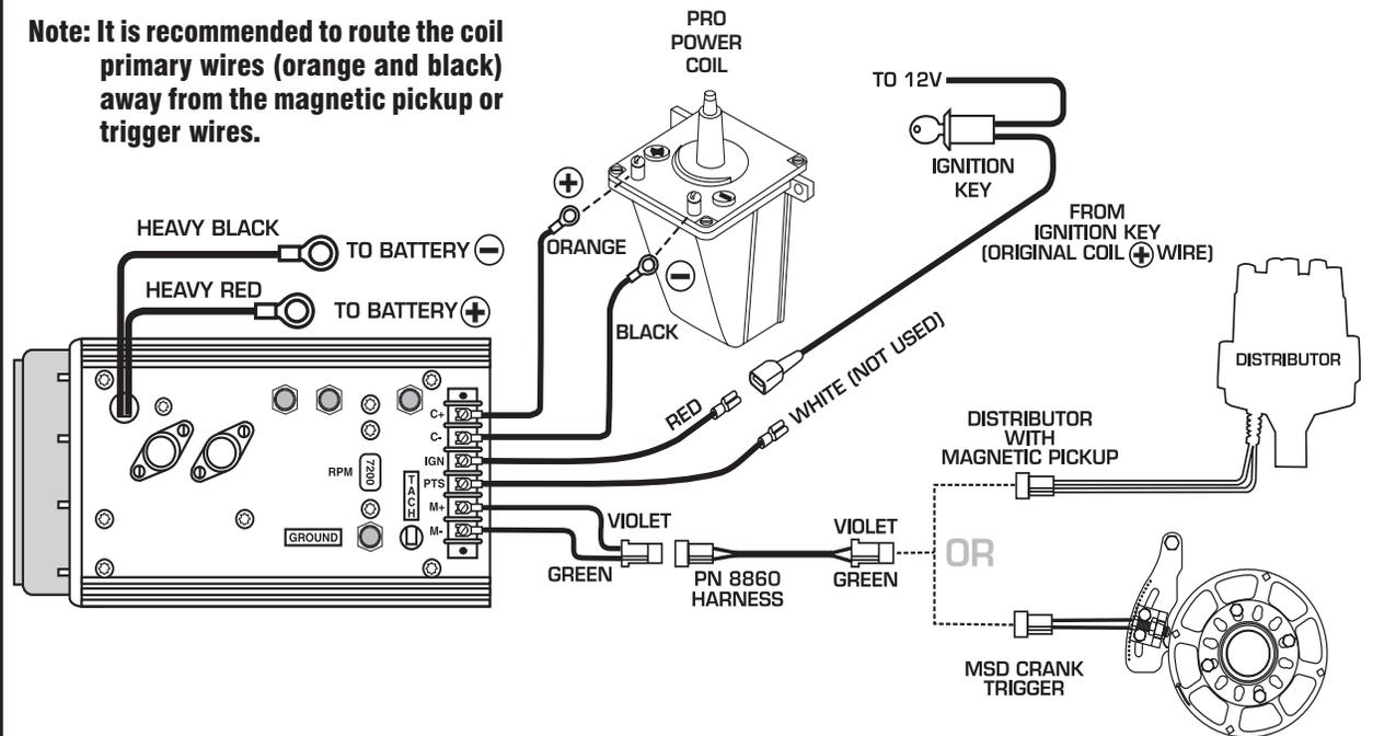
**Figure 3 Wiring the Pro Power Coil.**
