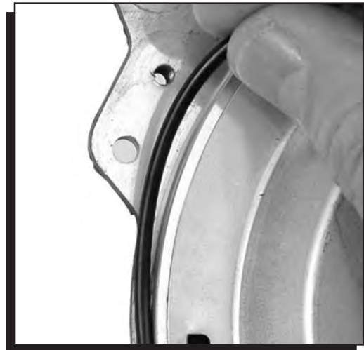
Figure 2 Installing the Distributor-to-Isolator Seal.
