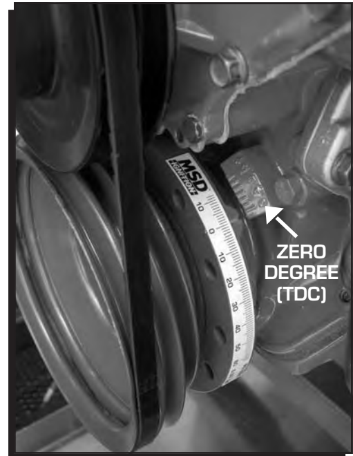
Figure 8 The Timing Tape Installed.
